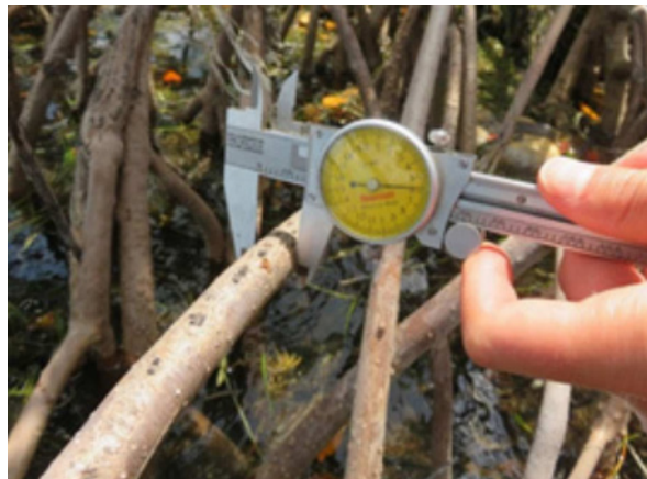
Figure A-5. Root diameter measurements using a caliper. (Photo by Tori Tomiczek and reproduced from Tomiczek et al. 2019, 1000.).
