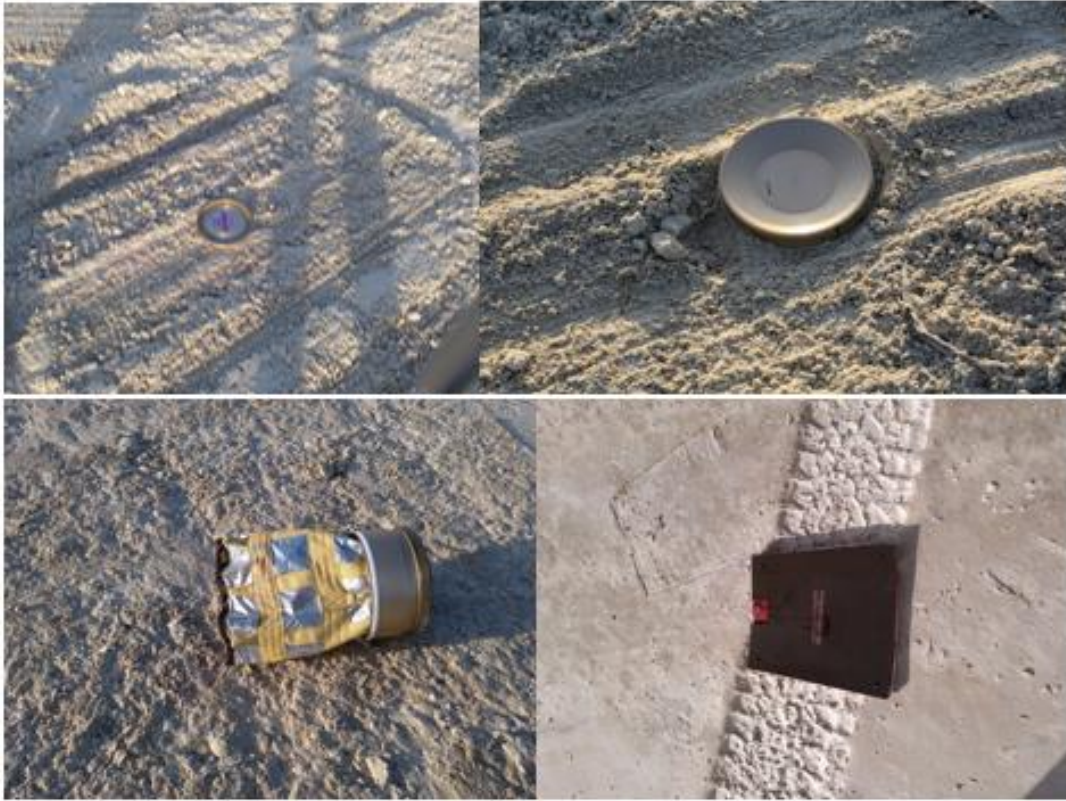
Figure 3-6: Mortar Lid, Sabot, and Forward Heat Shield Door Impacts
