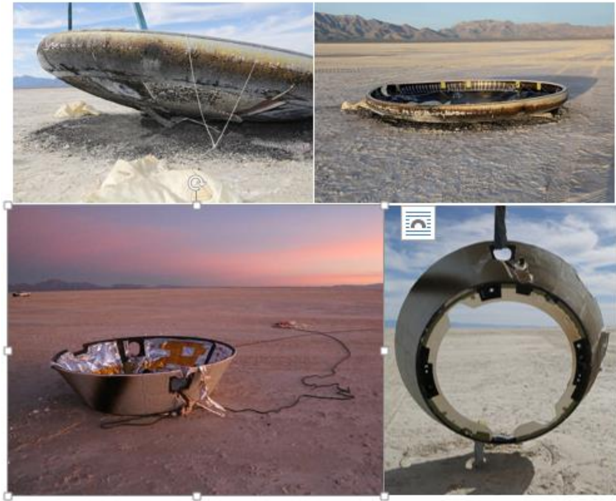
Figure 3-5: Base Heat Shield and Forward Heat Shield Impacts
