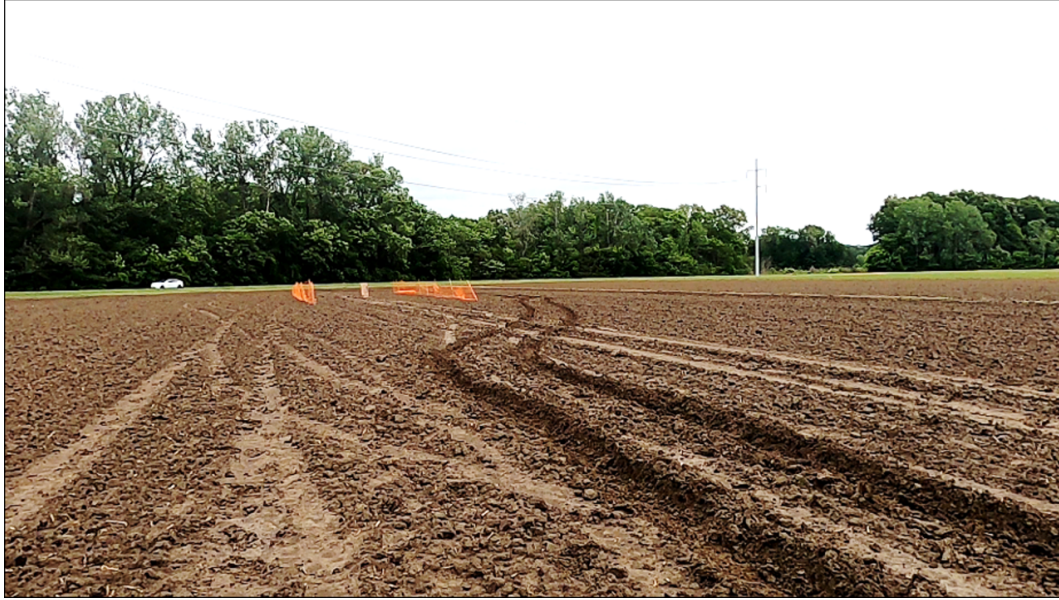
Figure 14: Deep ruts in the soft soil test area
