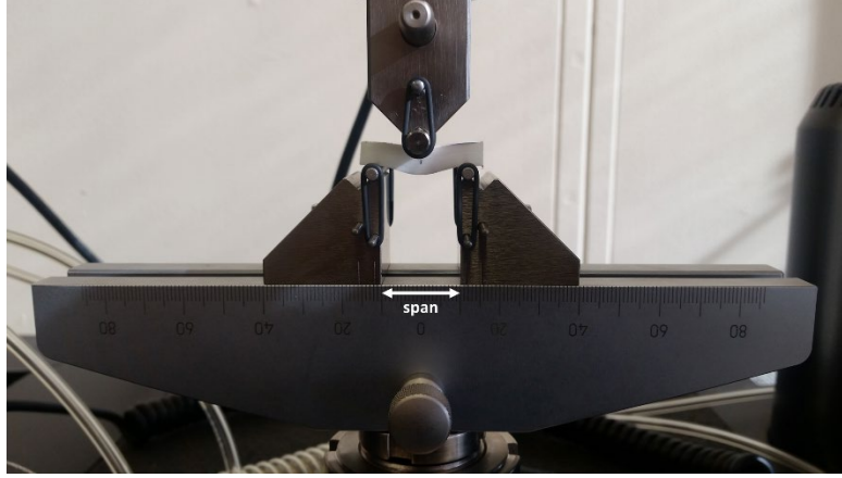
Figure 1 - The Instron flex fixture with short beam shear head
