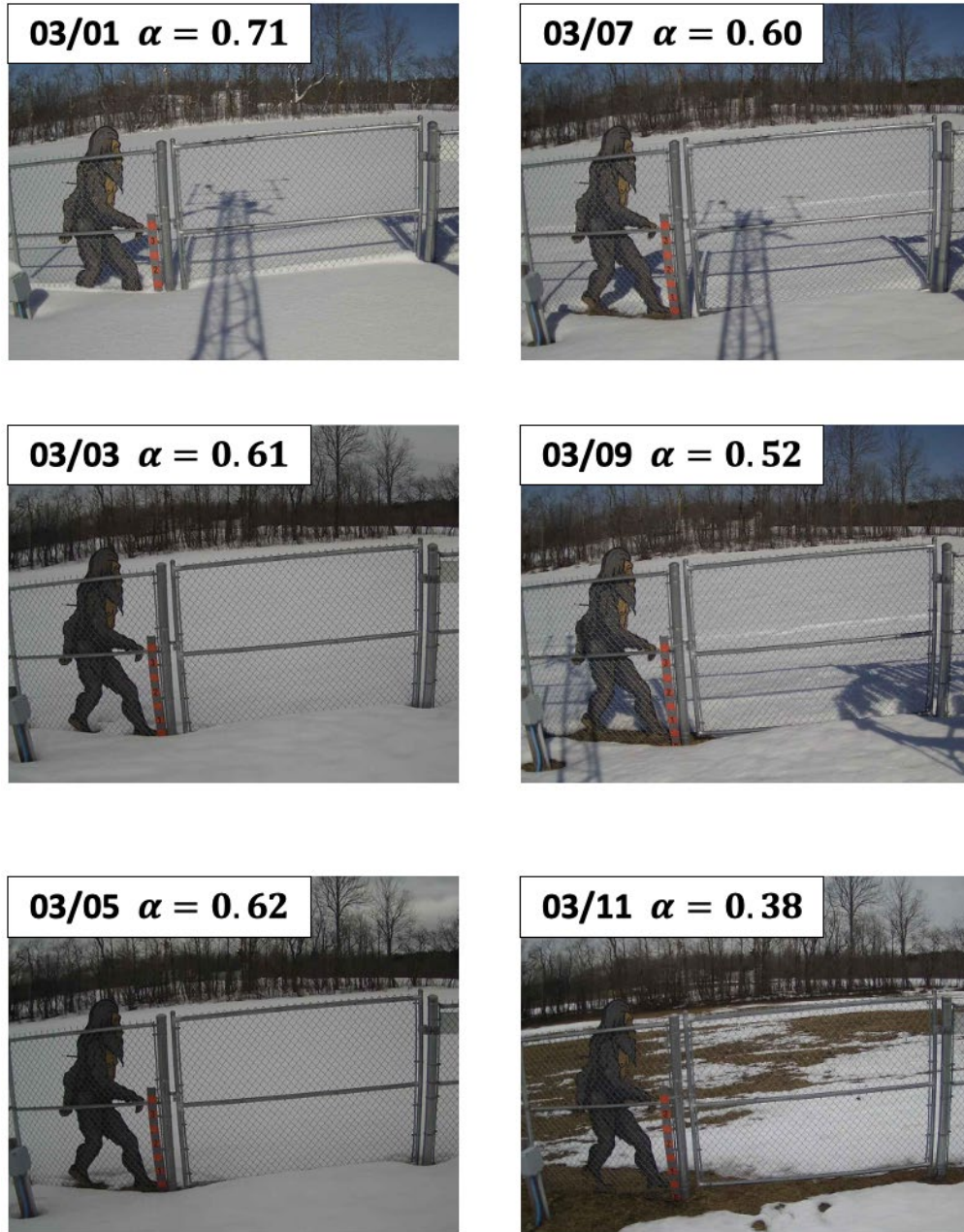
Figure 19. Automated site photographs from the Redfield site corresponding to the markers in Figure 19. Each image is taken at 11:55 a.m. local time. The measured daily median albedo is shown in each panel.
