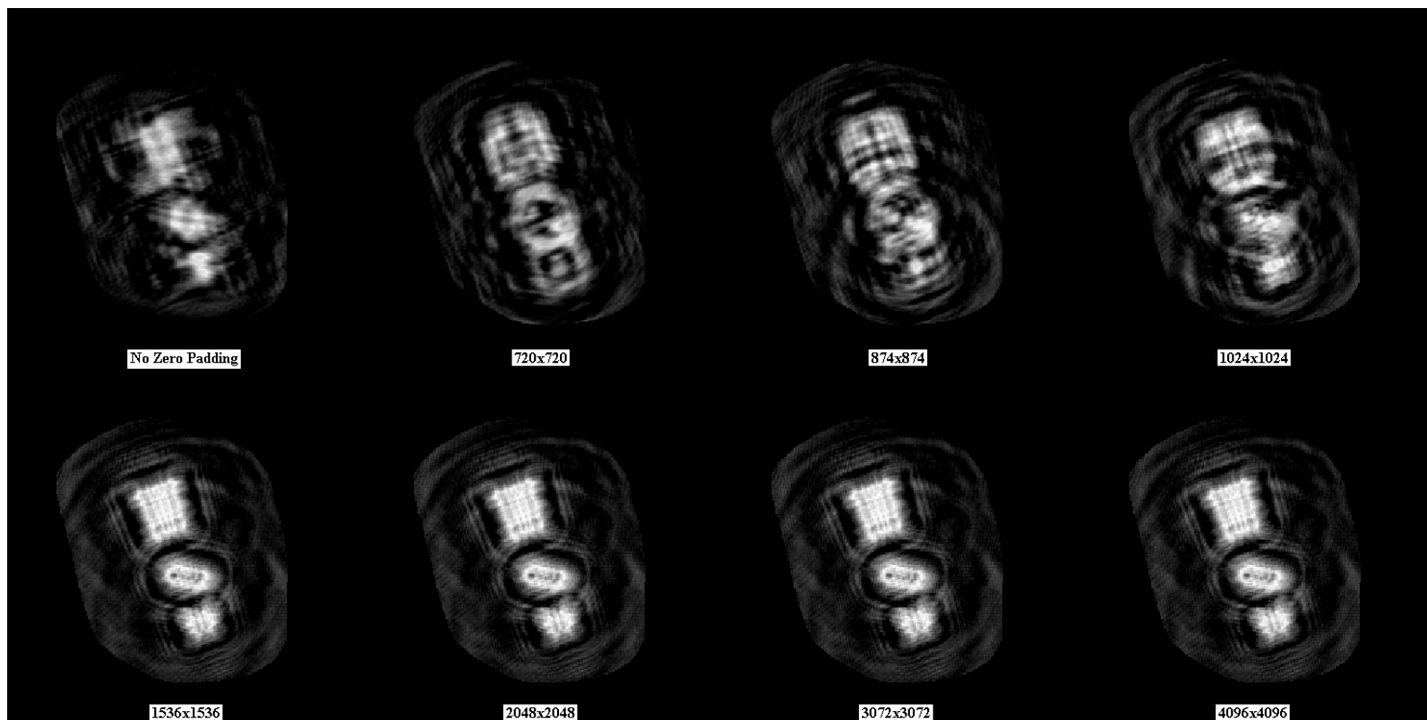
Figure 15: Silhouette reconstruction of the GPS satellite at 53.8 mm (5340 km altitude equivalent) using eight different amounts of zero padding, shown below each reconstruction.
