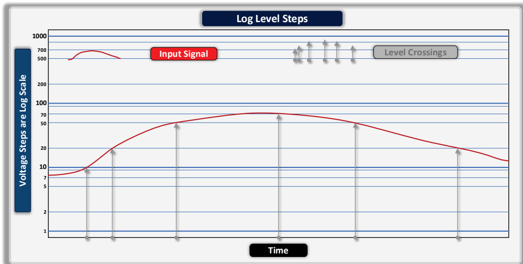
Fig. 26 Log level steps. Level-crossing ADC with log level steps.
