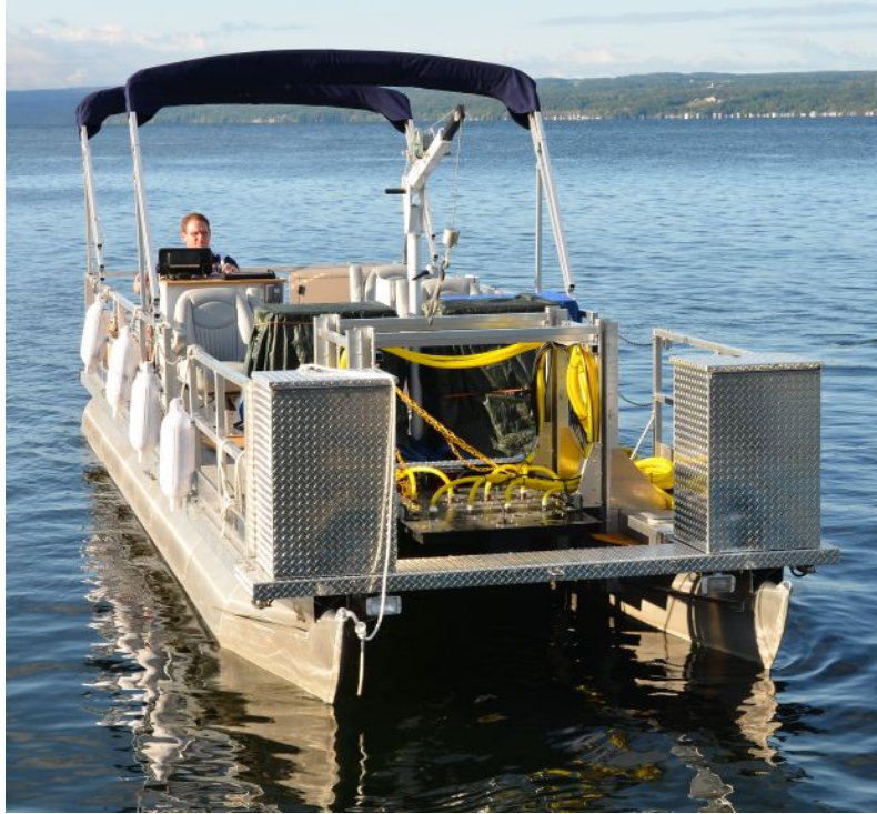
Figure 16: The Sound Hunter test platform is a nine-meter pontoon boat. The projector and receive array are shown here mounted in the forward portion of the boat. These components are mounted in a rectangular frame that is lowered into the water during testing.
