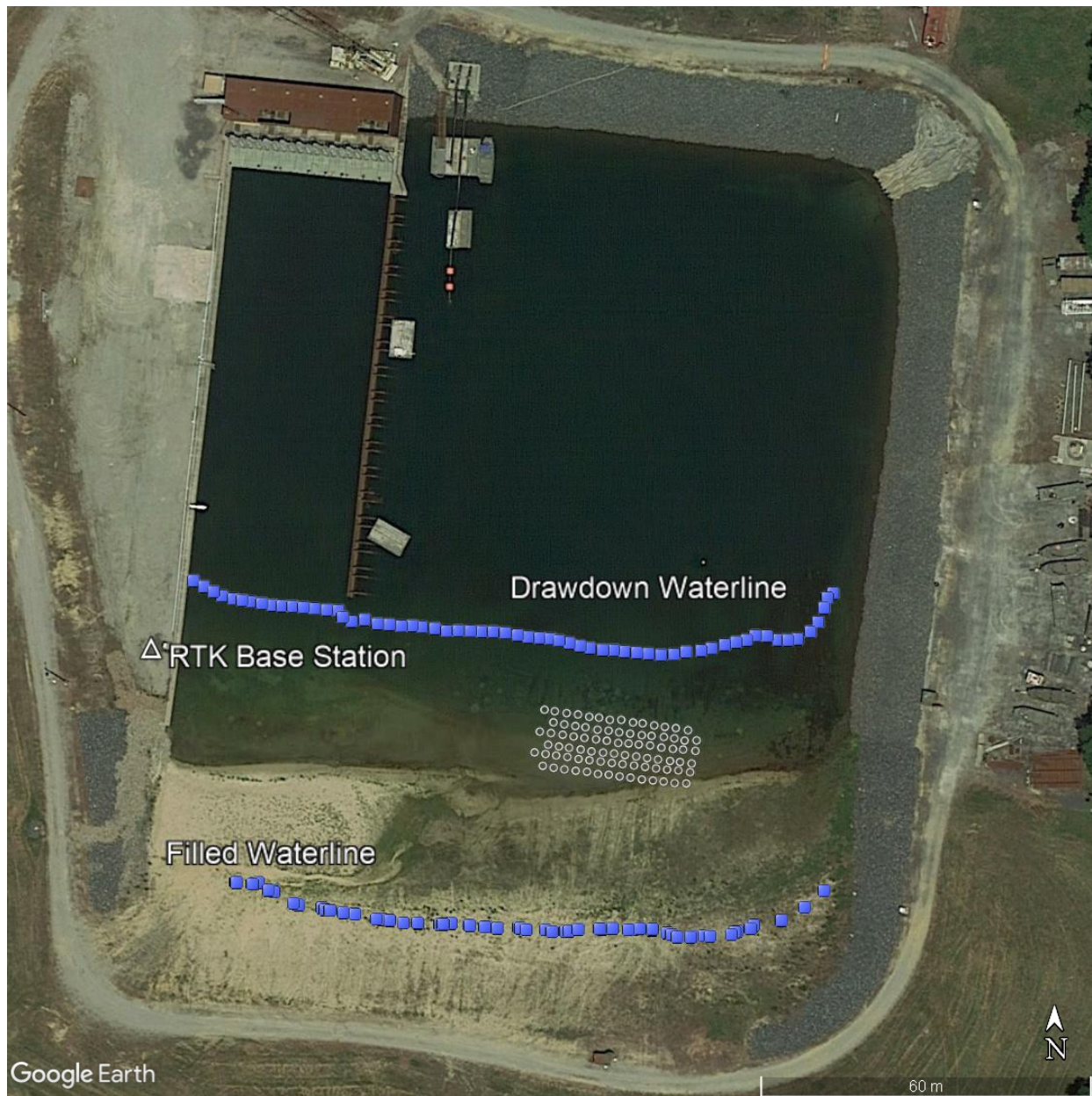
Figure 44: The targets described in Table 6 were installed into the LWE at the locations indicated by the white circles in this figure. During the installation of these targets the LWE water level was lowered to the draw-down waterline, which is shown by the northern line of blue squares. During testing the water level was raised to the filled waterline, which is shown by the southern line of blue squares.
