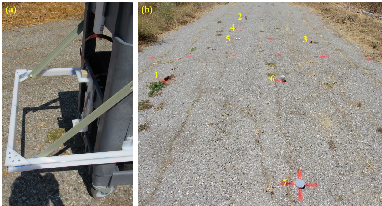
Figure 74 (a) MFAM sensor configuration for the low frequency AC field excitation method. (b) Survey site with targets. Compared with the site in Figure 72, 5 more targets were added. Among them, four are made of aluminum.
