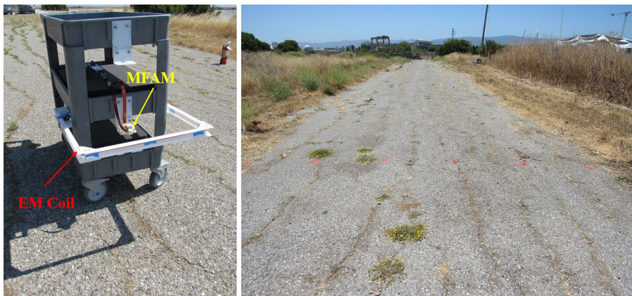
Figure 7 Combined MFAM-EM transmitter system and NASA field testing site.
