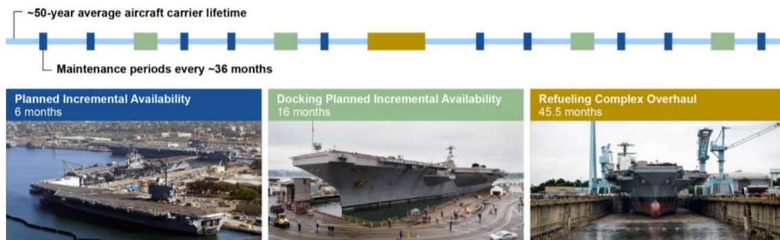
Figure 8. 36-Month Aircraft Carrier Maintenance Cycle over the 50-Year Expected Service Life 88
