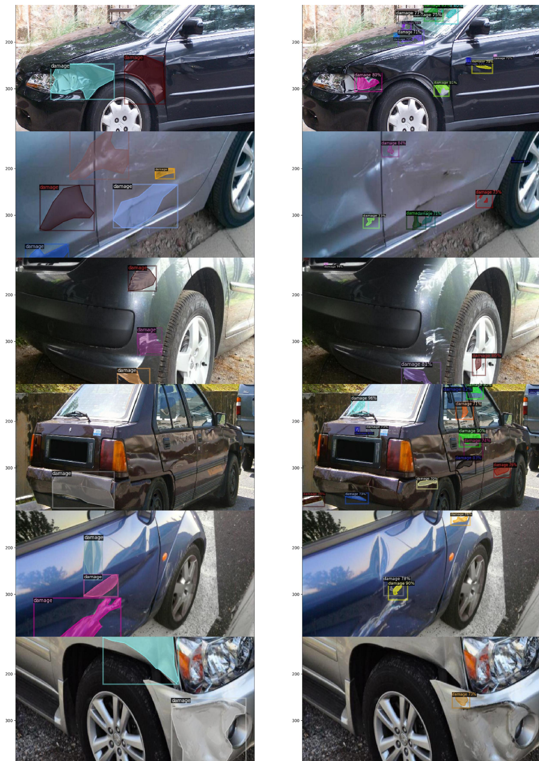
Figure 45: Examples of ground truth references (left column) and iteration 1500 Stage 3 model predictions (right column) of the real-world car damage data
