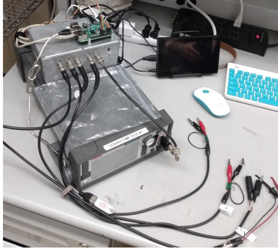
Fig. 5 The Raspberry Pi, Keithley 2450 sourcemeter, and splitter box are shown; all are attached to a compact 7-inch display
