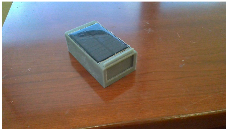
Fig. 1 EH sensor (3 × 5 × 2 inches with PV power source)*
