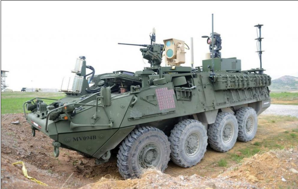
Figure 6. The Mobile Expeditionary High-Energy Laser Attached to a Stryker-Armored Vehicle
