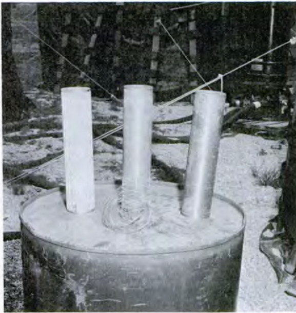
(Left to Right: Basic Septum Core; Septum partially wound; Septum as used in filter.)
