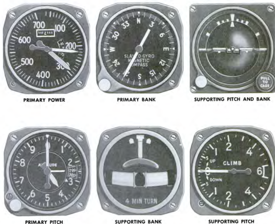
Figure 4-12. Flight Instruments in Straight-and-Level Flight.
