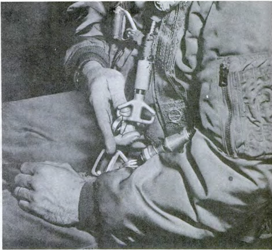
Figure 16-7. Method of Attaching Lanyard Hook to Ripcord Grip.
