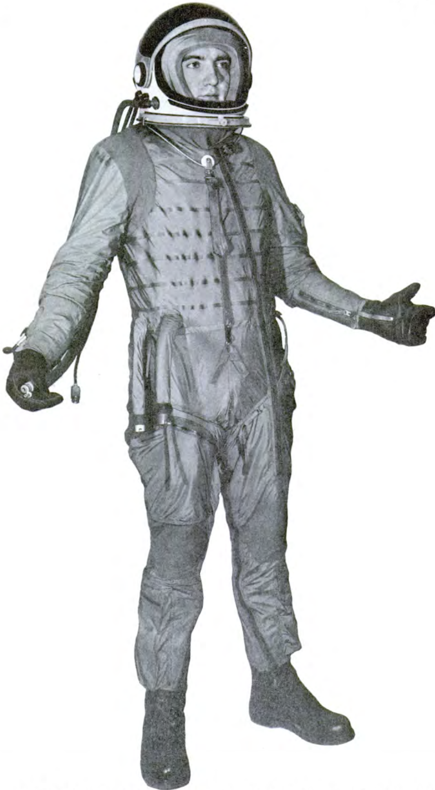
Figure 18-3. CSU-4/P Bladder Pressure Suit With HGU-8/P Helmet and MG-1 Gloves.
