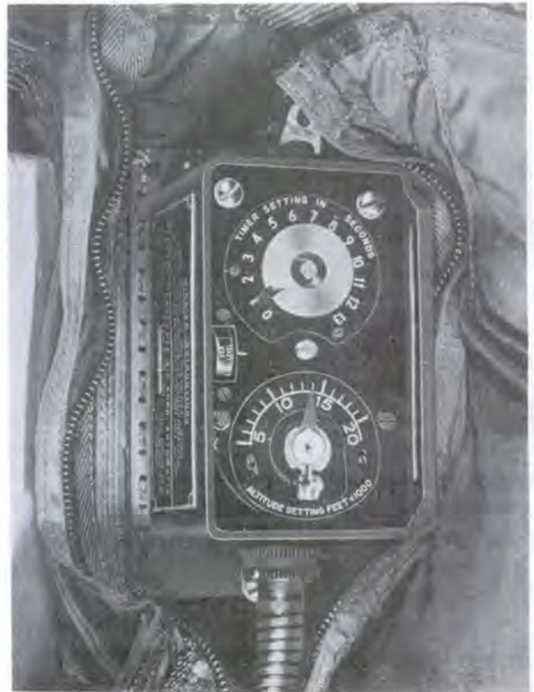
Figure 16-4. F-1B Automatic Parachute Ripcord Release, in the Latest Back Type Parachute.
