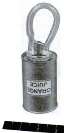
Figure 13-6. Experimental Can-Piercing Drinking Device Showing "Closed System" Looped Drinking Tube for Equalizing Pressure Within Can.
