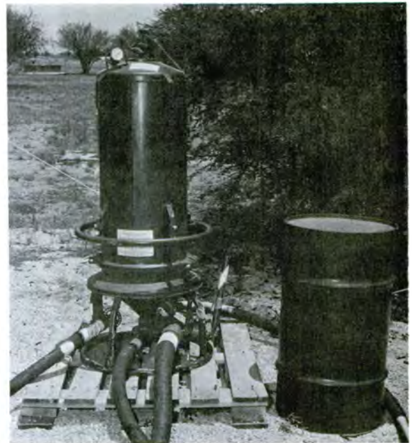
Figure 22-4. Diatomaceous Earth Filter Unit With Precoating, Influent and Effluent Lines.
