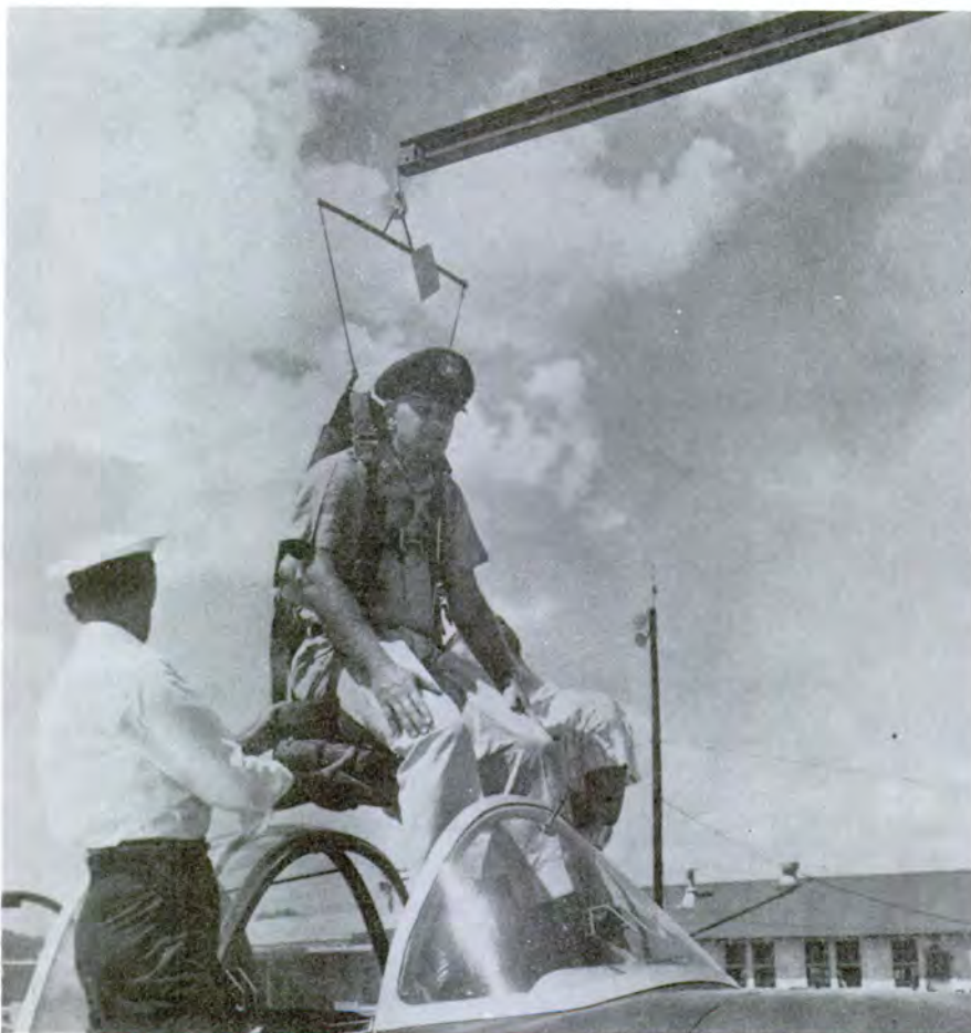
Figure 4-28. Demonstration of Sling Harness Used in Lifting a Back-Injured Pilot From the Cockpit. The Parachute Is Used To Stabilize and Support the Back.
