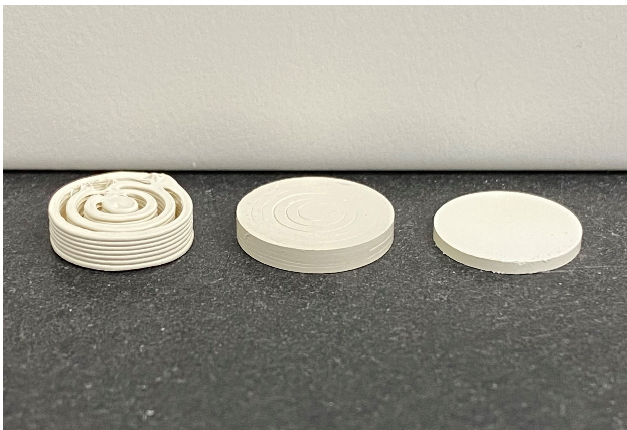
Figure 1. Disc preform consisting of concentric rings (left), disc preform after pressing (middle), and a disc pressed from PZT powder (right).
