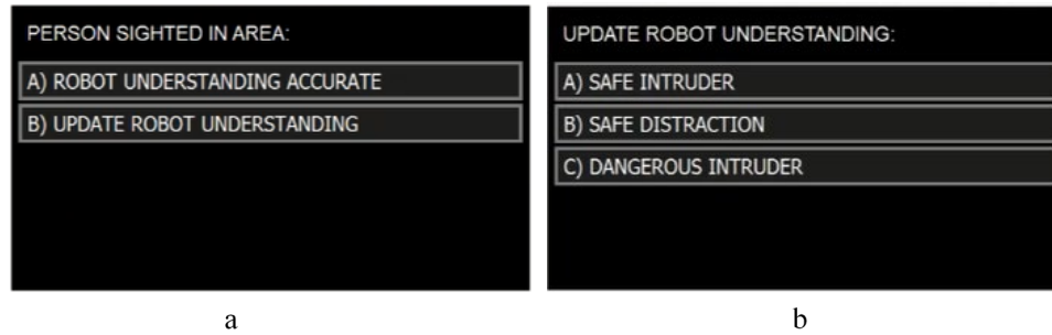
Fig. 4 (a) Bidirectional communications dialogue windows: when the robot identifies a person in the cordoned area, it asks if its assessment of the person is accurate; (b) if the participant indicates the robot's understanding is inaccurate, a selection of potential explanations is displayed
