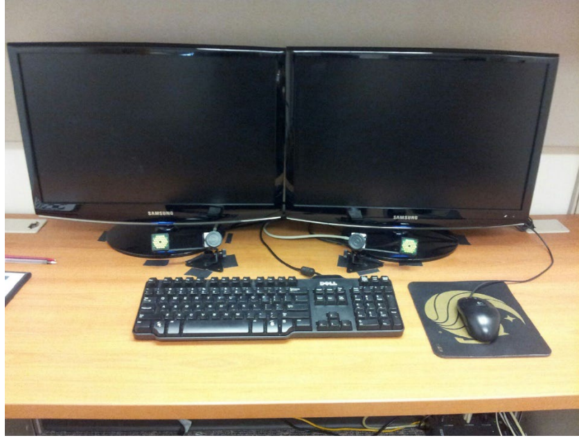
Fig. 3 Experiment station showing eye-tracking cameras positioned in front of monitors
