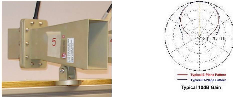
Fig. 23—The S-band horn antenna used for the far-field sources, and its typical principal-plane patterns
