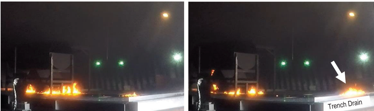
Figure 16. Re-ignition of Fuel vapors on the ILDFA
