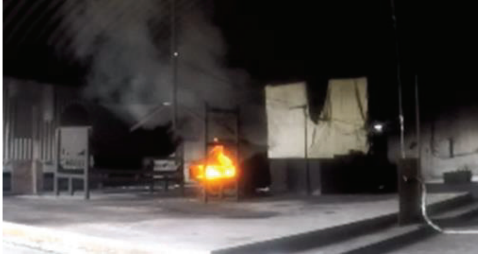
Figure 9. Fuel “Pre-burn” Before Fuel Spill on Concrete
