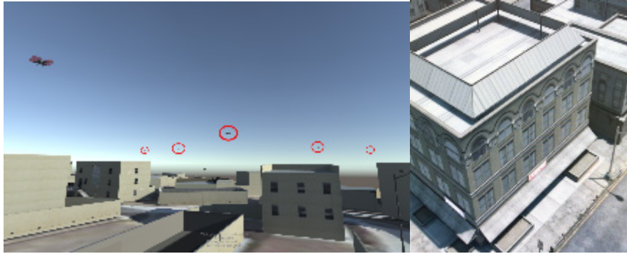
Fig. 39 (Left) shows a configuration of aerial robots that are dedicated to ensuring communication among the defense team. These agents leverage a connectivity maintenance algorithm to constantly move in order to maintain connectivity among the task agents. (Right) shows the view of a building from a quadrotor.
