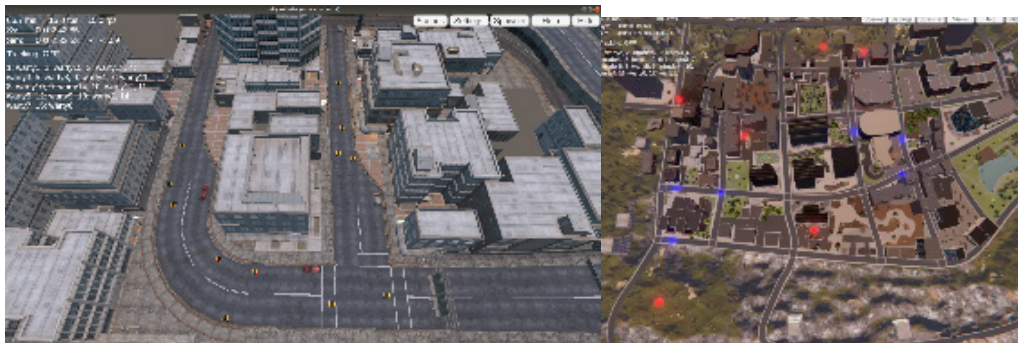
Fig. 38 (Left) Patrolling operations of 15 Warthog robots in the DCIST Unity simulation. (Right) Perimeter defense operations on two urban perimeters using six Warthog defender agents (blue) and six aerial intruders (red).
