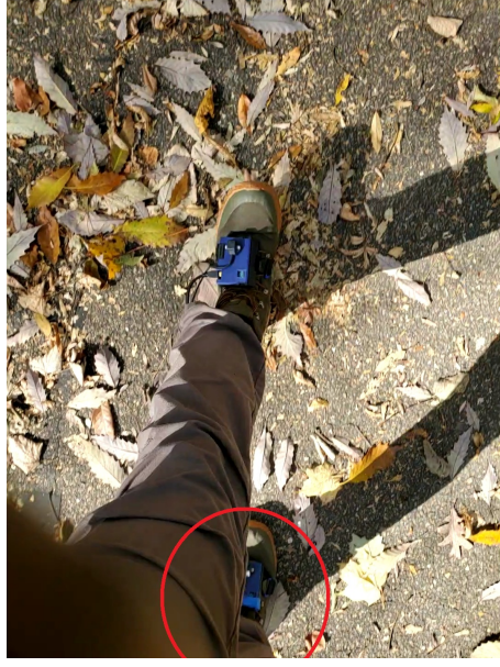
Figure 11: Walking, foot with zero velocity
