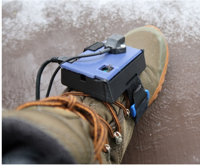
Figure 7: IMU and G4 sensor strapped to boot
