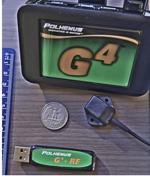
Figure 8: Polhemus G4 Sensor, transmitter, and receiver
