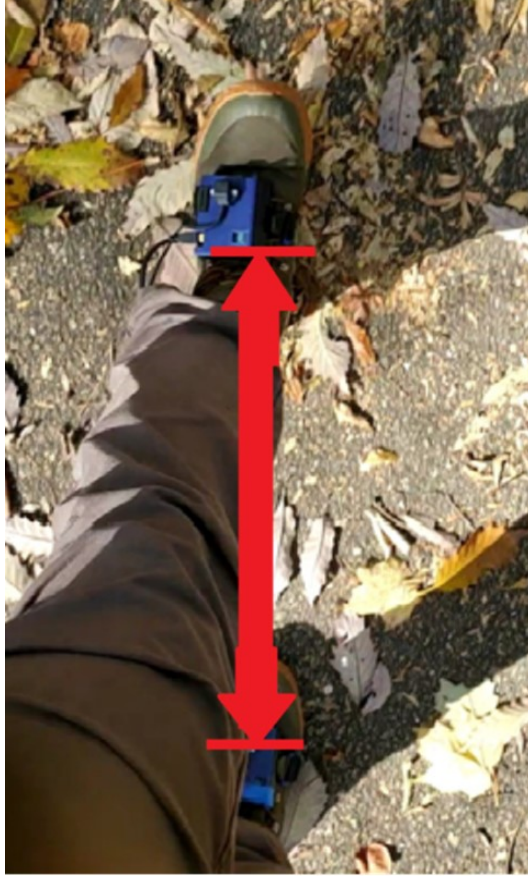
Figure 13: Walking, foot-to-foot ranging measurement
