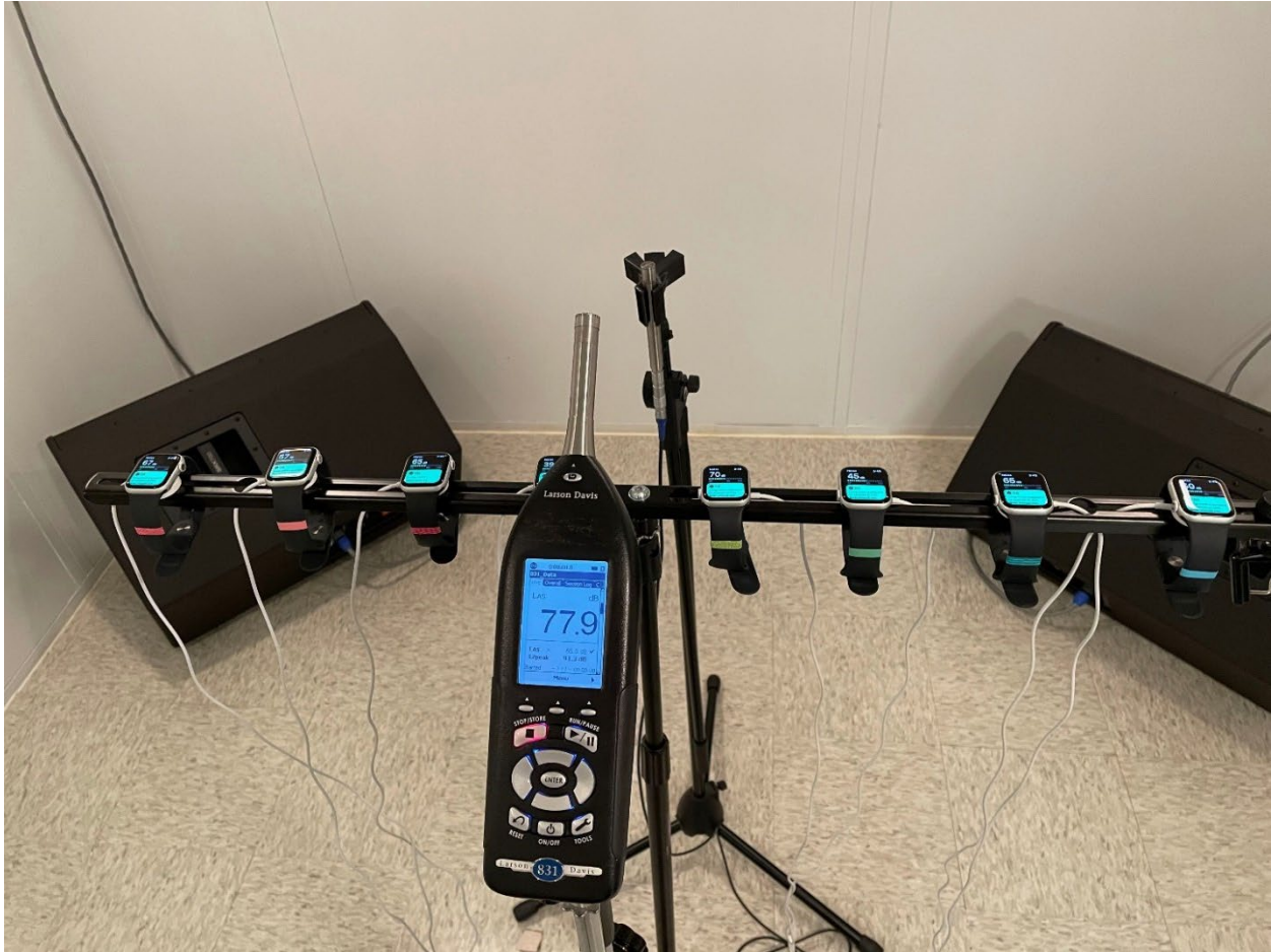
Figure 2. The testing apparatus consisting of a smartwatch stand, reference microphone and reference system and sound level meter. Noise generation speakers shown in background.
