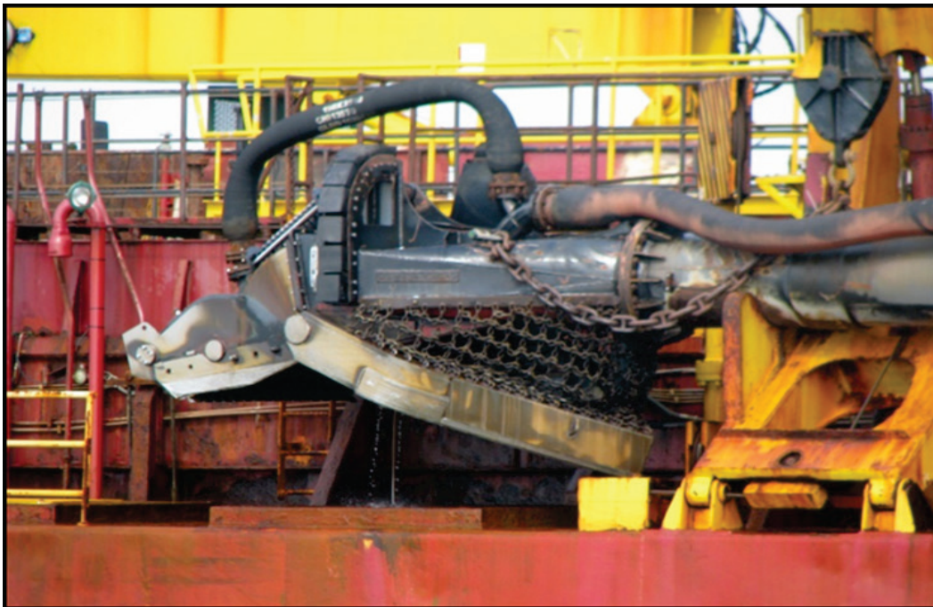
Figure 2-2. A draghead of a hopper dredge with a sea turtle deflector. Photo credit: USACE-ERDC.
