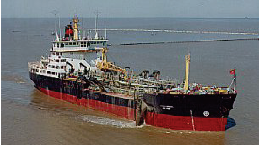
Figure 2-1. Example of a hopper trailing suction-type dredge. Photo credit: USACE-ERDC
