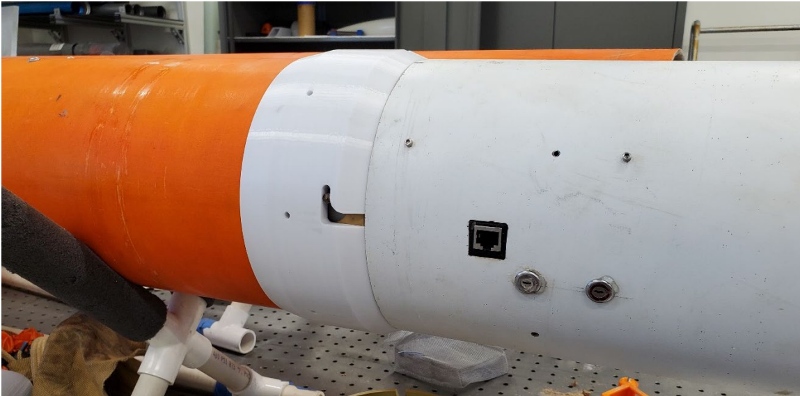
Figure 67. Polycarbonate Coupling Installed on Sled.
