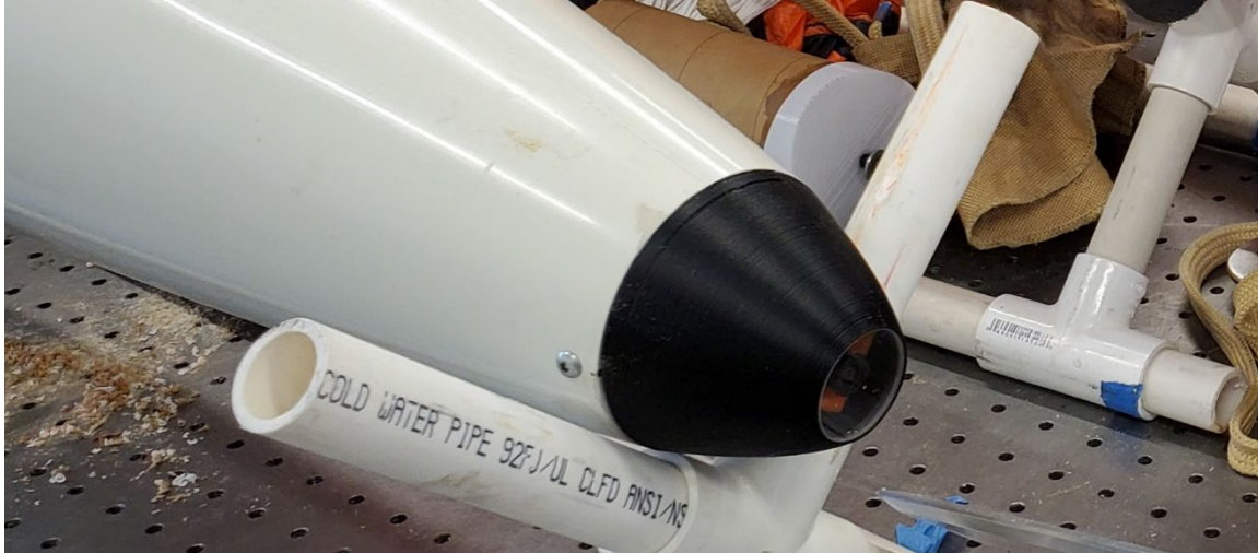
Figure 68. PETG with Carbon Nanotube Camera Housing.
