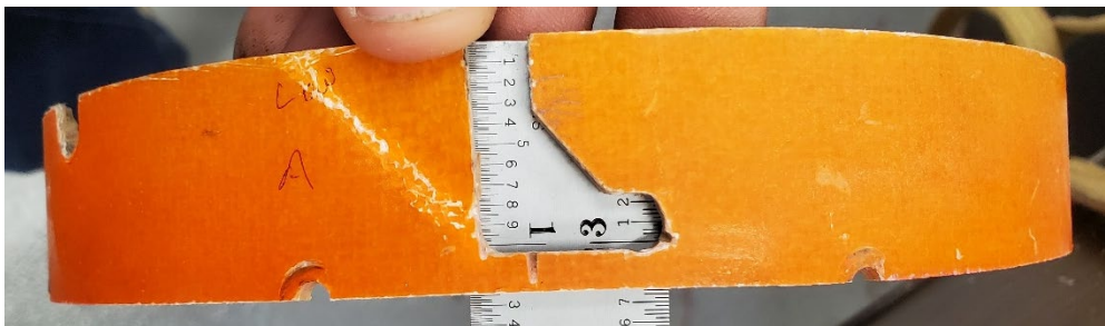
Figure 66. Damaged Sled Coupling Removed from Sled.
