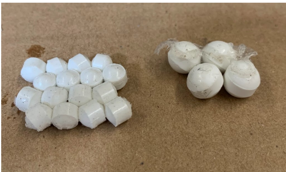
Figure 25. 0.635 cm and 0.952 cm \text{Al}_2\text{O}_3 ceramic spheres, both 90% alumina.
