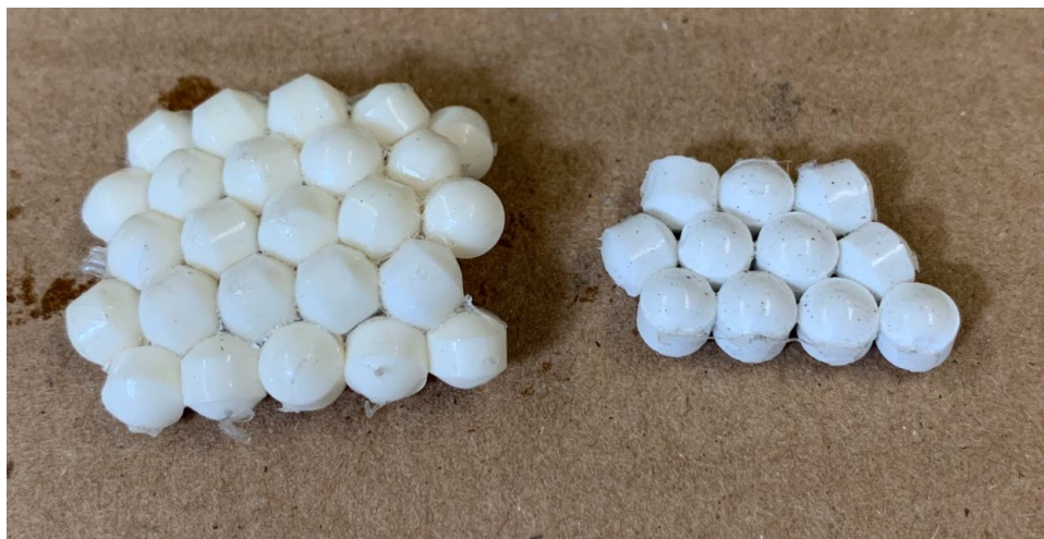
Figure 24. \text{Al}_2\text{O}_3 ceramic spheres of different alumina purities. Left is 99.5% alumina; Right is 90% purity.
