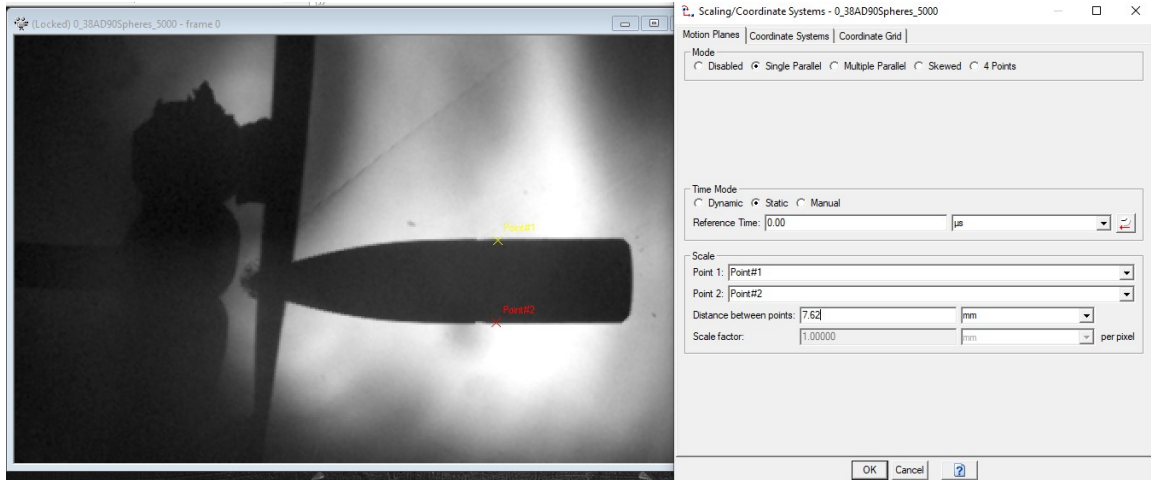
Figure 19. TEMA scaling setup.
