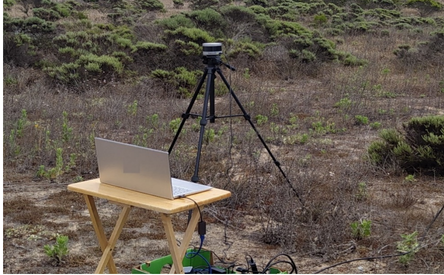
Figure 31. LiDAR sensor and some of the auxiliary equipment set up in the test field.
