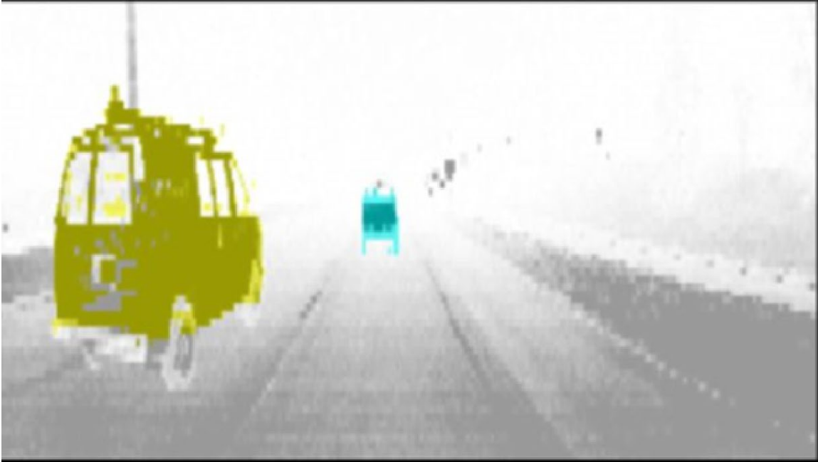
Figure 27. Semantic segmentation of point clouds. Adapted from [16] (colors inverted).
