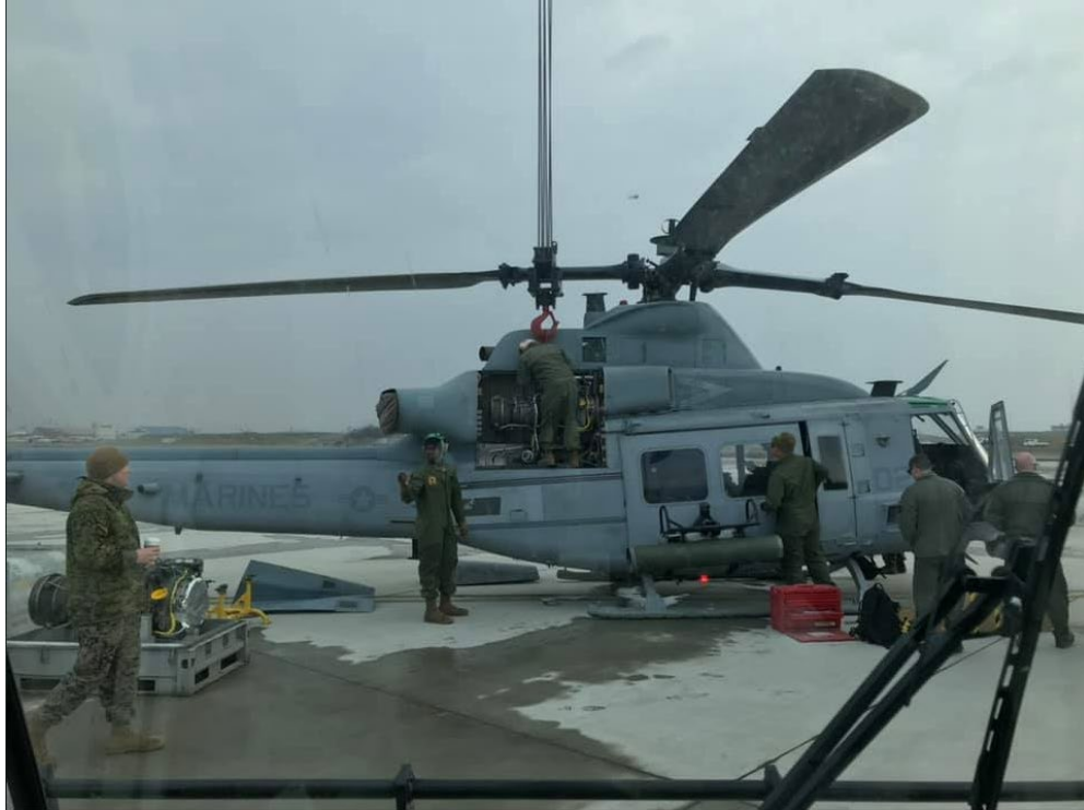
Figure 3. Engine Replacement Being Done on a UH-1Y Huey.
