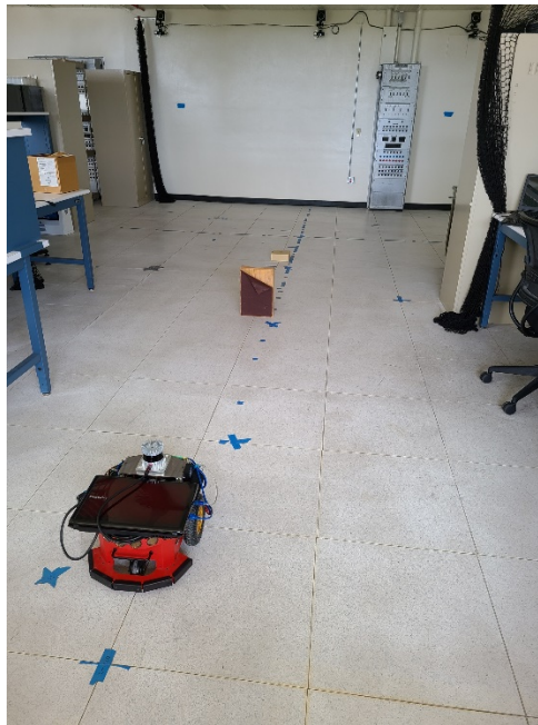
Figure 46. Experiment 3: Combined Obstacle Detection and Avoidance
