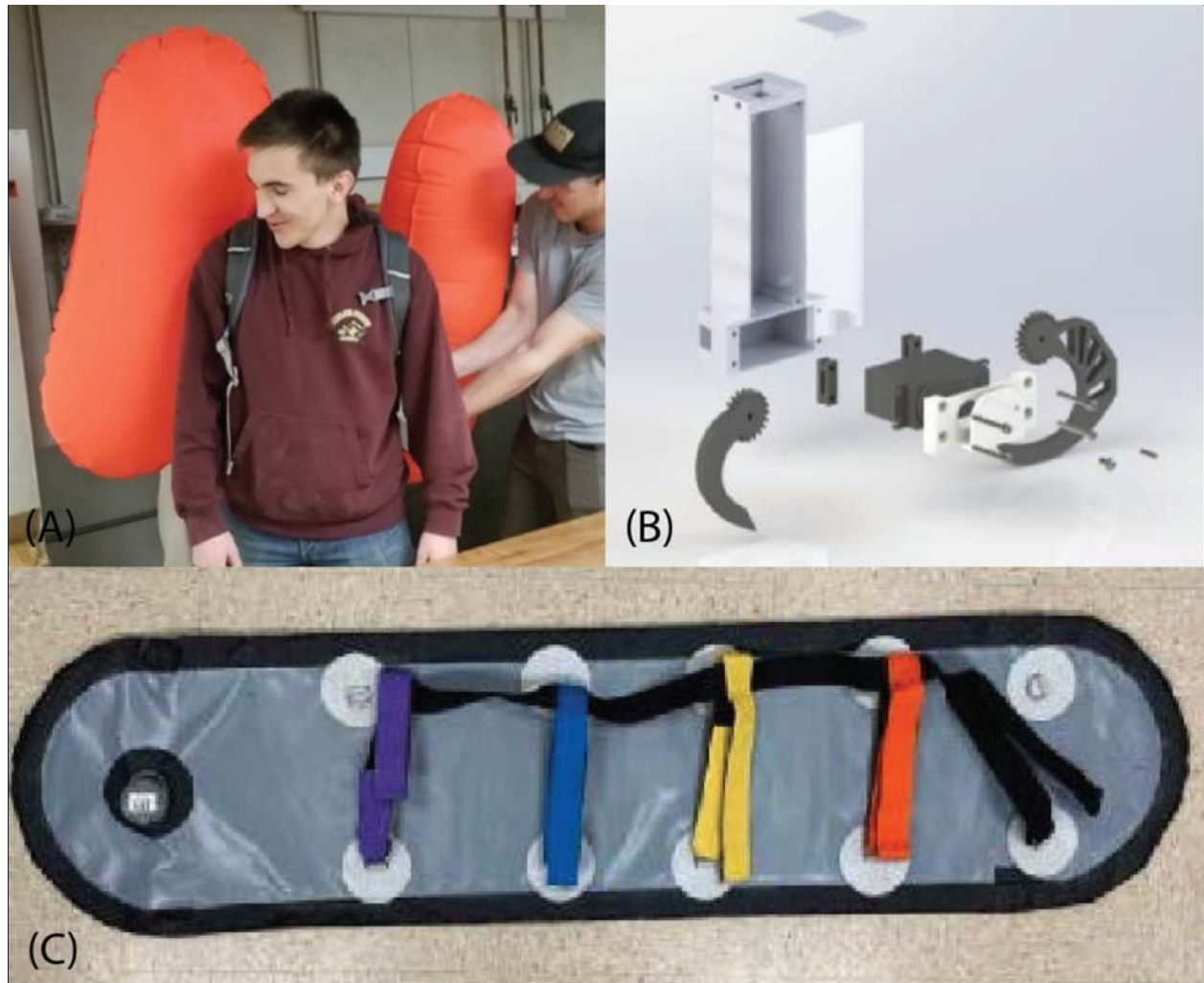
Figure 11. (A) UG team test their prototype for the AvyPouch system, (B) Exploded view of the FAAST teams' claw design using a single servo to drive a double gear that holds a 5 kg payload, and (C) Final prototype strap system for a collapsible search and rescue board.
