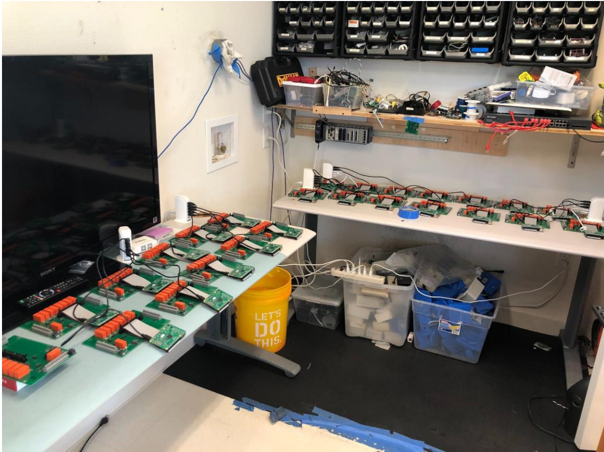
Photographic evidence of 24 HVAC and 3 EVSE follower boards connected in the PSI lab for communication testing, using data from PSI's participant network.
