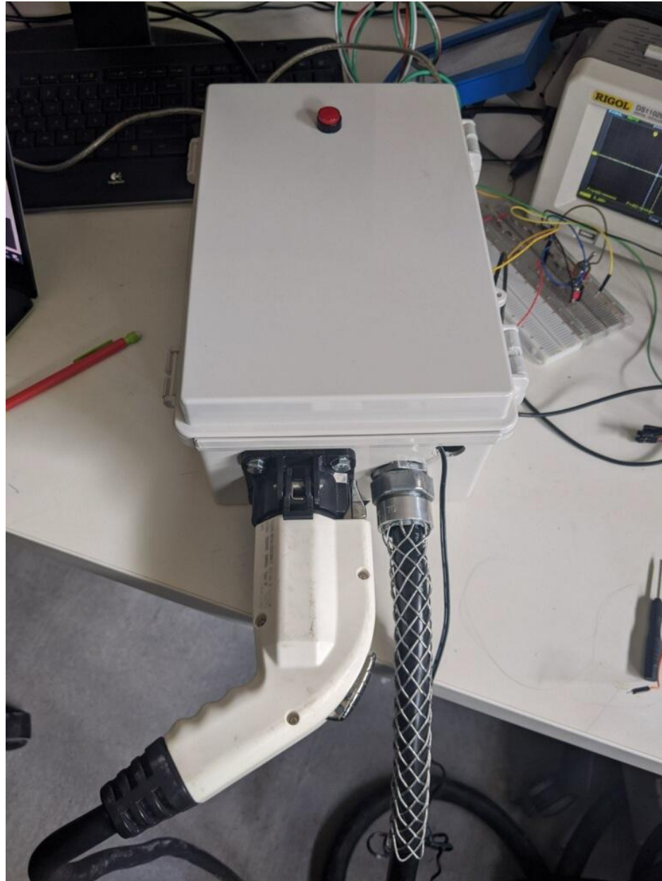
Photographic evidence of the EVSE test set at the PSI lab, including EVSE follower and J1772 connector
