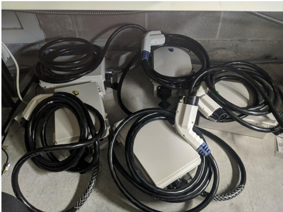
Figure 10: Photographic evidence of five sets of fully assembled EVSE Controller board connected to J1772 compatible connector
