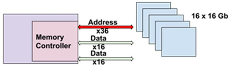
**Figure 3. Memory design using 32 x 2 GB DRAM chips**
