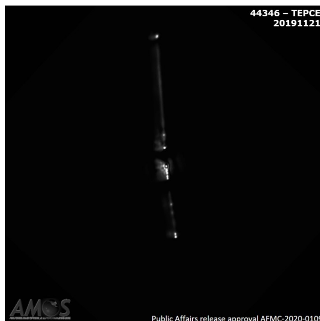
Fig. 40—Image of TEPCE after tether deployment taken at the Air Force Maui Optical and Supercomputing (AMOS) site
