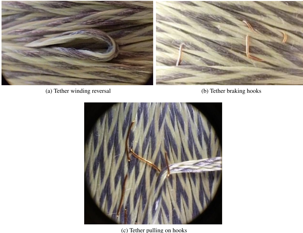
Fig. 15—Tether Winding Details
