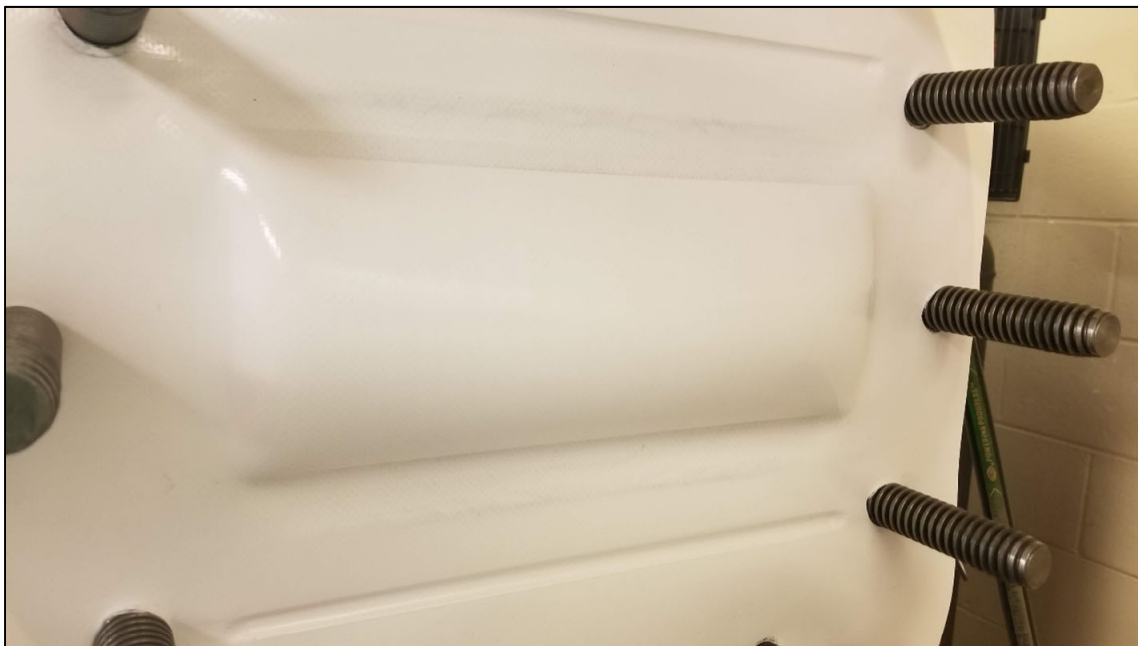
Figure 8. Failure of rupture of high tensile strength Mylar membrane in our blast simulator (Ora Inc). Note that the membrane was deformed (stretched) but did not rupture in our system that uses compressed gas to pressurize the compression chamber.
