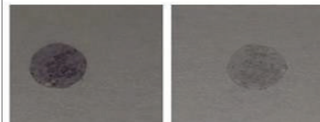
Figure 16. Photographs after exposure for concentration runs 1–8, blower (left side) versus pump (right side). Visual inspection of color profile shows the fan housing performed better than the intake approach for the eight trials tested.
