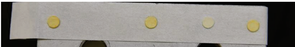
Figure 37. Three VX dots were exposed to VX in the chamber for a total of 100 min. Concentration of chamber was 0.056 \text{ mg/m}^3 at 100 min. Slight color change was observed when an unexposed dot was placed (third from left) for contrast.
