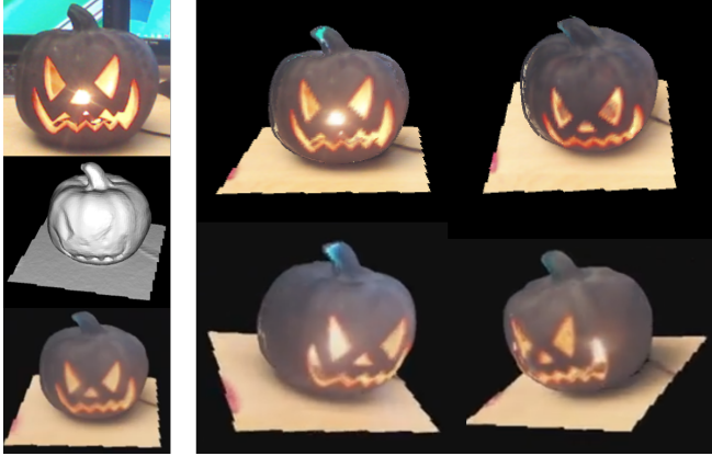
Fig. 5. (top left) An image of a real object captured using a Kinect v1. (middle left) The untextured 3D model. (bottom left) The model with a fixed texture generated from blending the source images (right). The model with view-dependent texture rendered from several viewpoints. Note the flame from the candle within the object.
