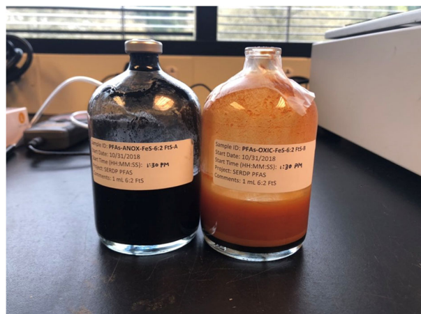
Figure 2.7 Anoxic (left) and oxic (right) FeS-amended bottles. Clear visual evidence of FeS oxidation in the presence of oxygen was observed.
