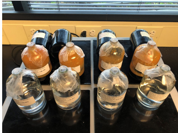
Figure 2.6. Experimental serum bottles filled with ferrous minerals, clays, or neither (controls).
