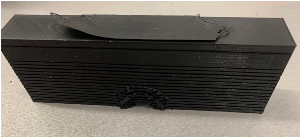
Fig. 12 3D printed target block with unwanted horizontal bands
