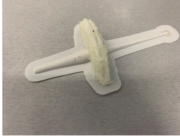
Fig. 10 Jet formation at a later timestep with PVA supports and a PLA raft to ensure the print adheres to the print surface
