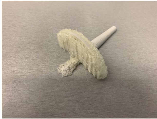
Fig. 8 Jet formation with PVA support
