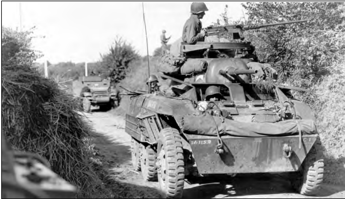
Figure 3. Cavalry Vehicles: M8 Light Armored Car (foreground) and Half-Track (background) in Belgium
