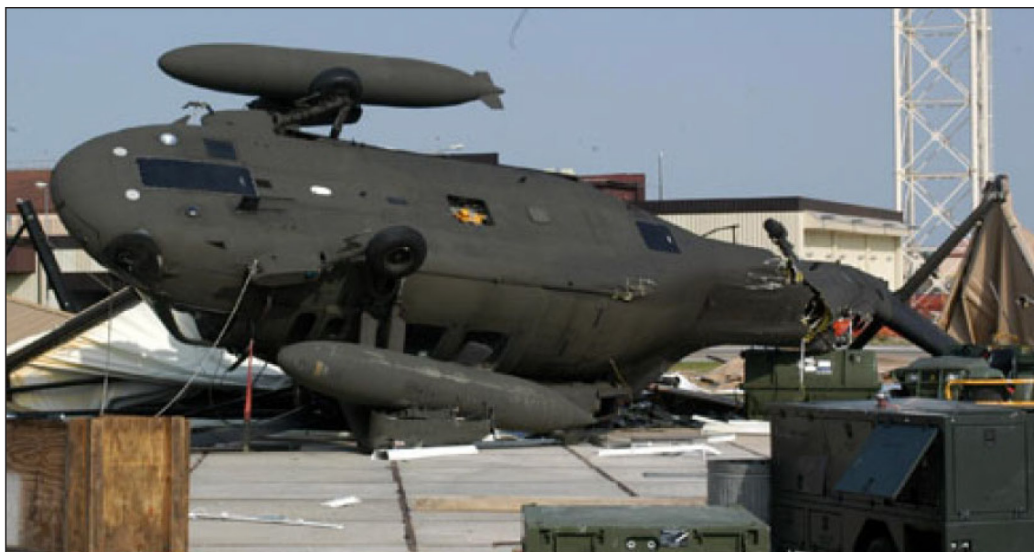
Figure 5: Helicopter Damaged by an Extreme Wind Storm at a Department of Defense Installation in Europe
