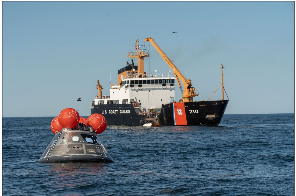
Figure 6: Orion Crew Module Test Article
