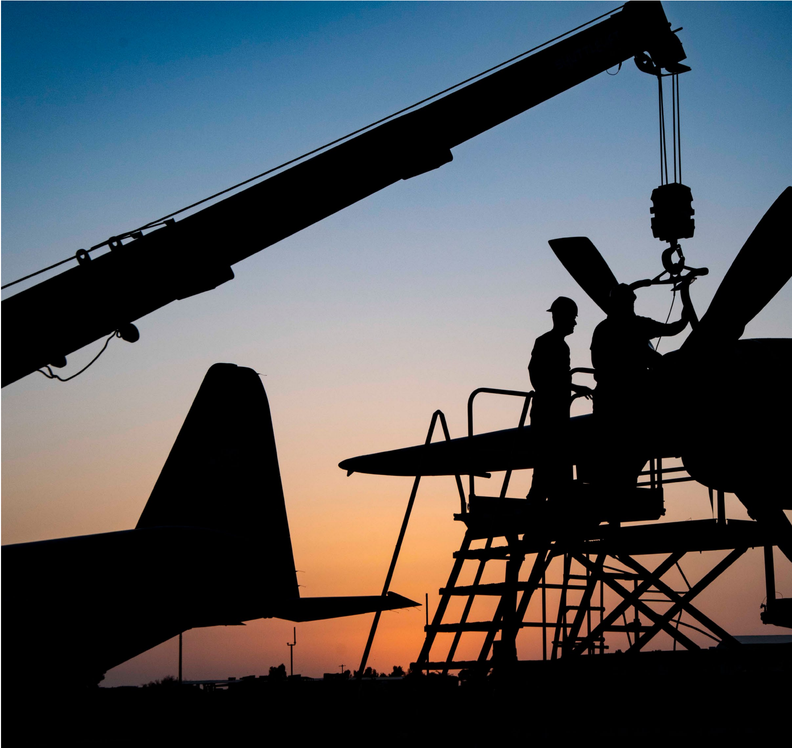
Crew chiefs assigned to the 386th Expeditionary Aircraft Maintenance Squadron “Blue” Aircraft Maintenance Unit perform a C-130 Hercules propeller swap Ali Al Salem Air Base, Kuwait, June 25, 2020. (U.S. Air Force photo)
