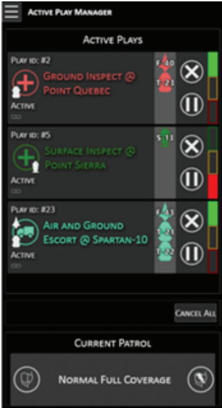
Figure D.4. Active Play Table HMI. Each row provides additional information on plays under way as well as the ongoing patrol. For each play, the row shows (from left to right ) the type of play, play location, assigned vehicles, functionality to cancel or pause the play, and a color indicator of the progress of the play. Selection of the row calls up the corresponding Workbook (e.g., to modify the play), including the Play Quality Matrix of figure D.5.
