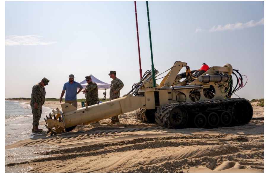
Photo: Mini Robotic Submersible-Dredge was developed by the military for digging out and removing underwater sediment to support amphibious assaults, but it can also be used for water resource management applications, such as navigation channel maintenance
