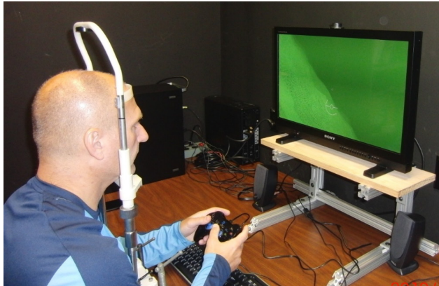
Figure 14. Experiment 1 set-up. Participants sat 57 cm from display with an eye height aligned to the center of the display. Their head was stabilized in chin and head rest. Here the participant is 'flying' an aircraft while observing the corresponding ASAR attitude representations.
