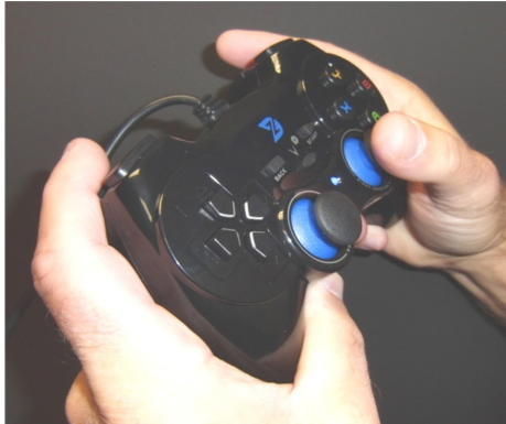
Figure 15. Experiment 1 input device. Participants entered their inputs with a gamepad controller. The left hand index finger progressed the participant through the testing while the right handed thumb input the test responses.
