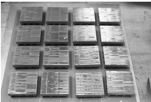
Figure 12. The sixteen EM susceptor tiles have 0.002 inch thick BNi-2 foil spot welded into the Gas Tube braze channels.
