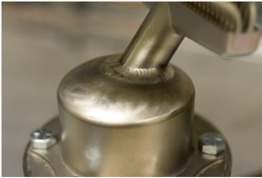
Figure 17. TIG welded joint between a Collector and a Piston Cylinder
