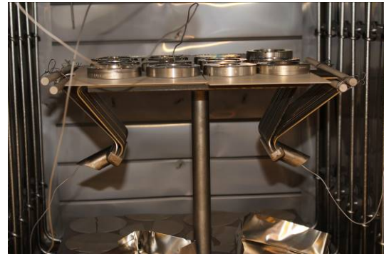
Figure 10. The clamps are replaced with additional Alumina plates and stainless steel weights to keep the tubes flat in the vacuum brazing furnace.
