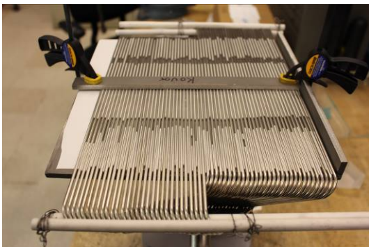
Figure 9. The Gas Tubing Array is clamped down to a Kovar setting plate with 0.020 inch thick Alumina strips separating tubes, and 0.020 inch thick Alumina plates between the Inconel tubes and the Kovar setting plate, also Alumina rods tied together with Molybdenum wire help align tube ends.
