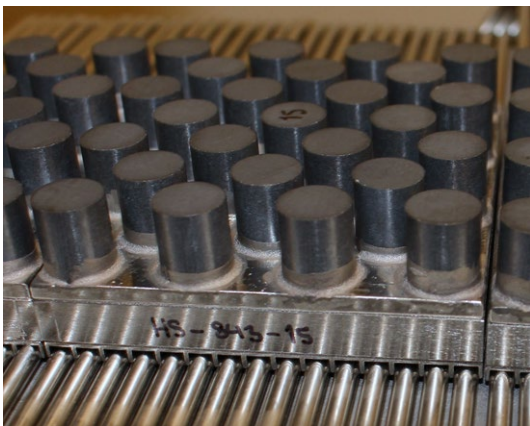
Figure 2. A EM susceptor tile. Visible are the 25 AlN Cylinders and metal baseplate.
