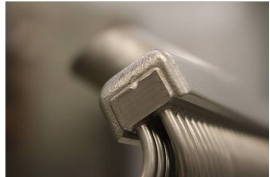
Figure 7. The rectangular Header block (center) is inserted in a channel machined into each Header. Also visible are the tack weld spot and the subsequently brazed joint.
