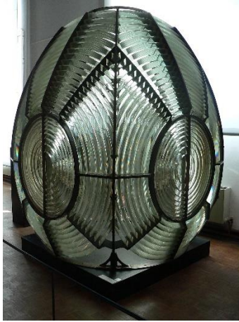
Figure 5. A large-diameter Fresnel lens used in a lighthouse. 24
