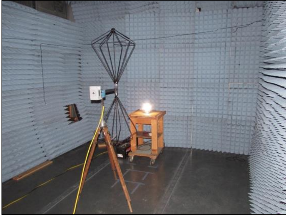
Figure 5. Radiated emissions test setup inside the chamber at IMANNA Labs.
