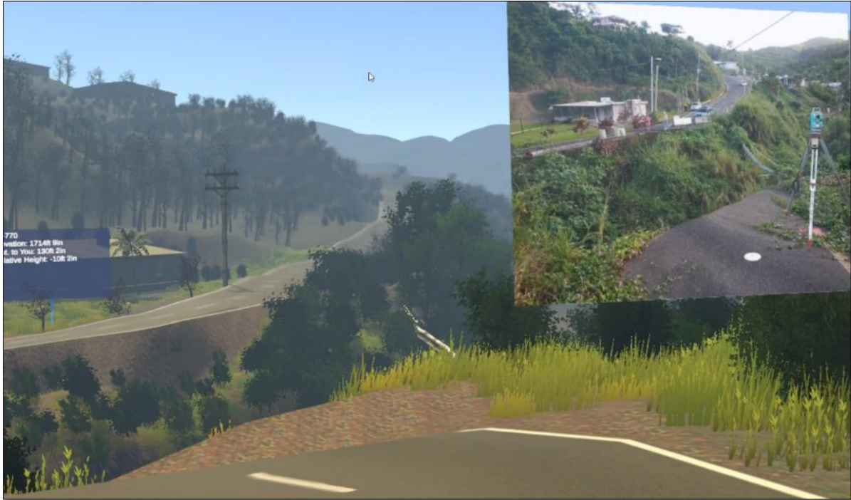
Figure 14. Virtual reality rendering of PR-770 damage area, showing a geotagged photo taken from the same perspective during an in-person site inspection.
