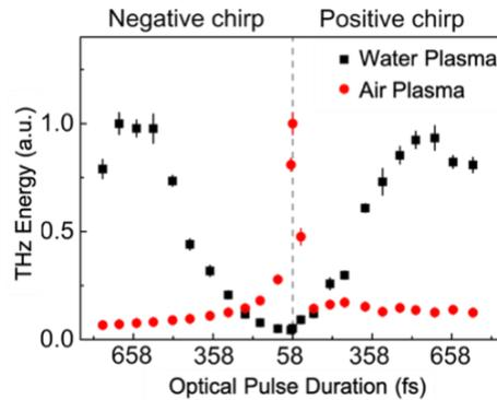
**Figure 7. Normalized THz energy with different optical pulse durations.** <sup>[10]</sup> THz signal generated by water plasma prefers an optical excitation with a longer pulse duration. However, the generation from air plasma is always in favor of the shortest pulse.
