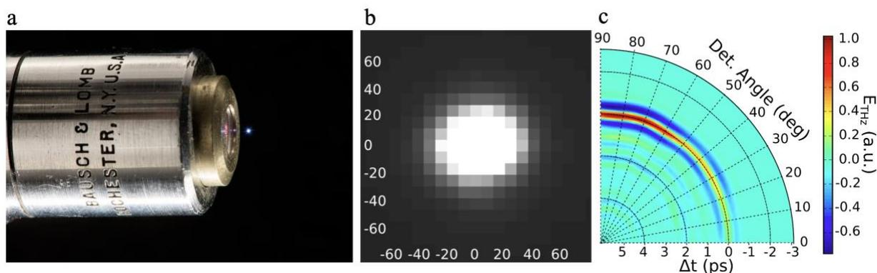
**Figure 4. Micro-plasma and the signal distribution.**<sup>[34]</sup> **a** A photo of the micro-plasma fluorescence obtained by focusing the laser beam with a high NA microscope objective. **b** A magnified image of the micro-plasma (unit is  $\mu\text{m}$ ). However, the plasma spot's contribution to the THz wave is about one  $\mu\text{m}$  or less. **c** Measured THz field as a function of the THz emission angle. The optimal angle is 80 degree from laser propagation direction.
