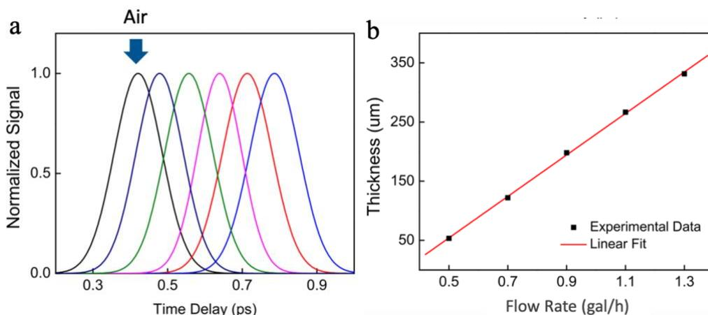
**Figure 3. Calibration of the water film thickness.** **a** The original (air) signal from the autocorrelation system is plotted in the black line. With the water film in one of the two beams of the autocorrelation system, the signal peak will move linearly with the increase of thickness. **b** The linear dependence of the thickness on the flow rate. The thickness of the water film can be continuously tuned from  $50 \mu\text{m}$  to  $350 \mu\text{m}$ .
