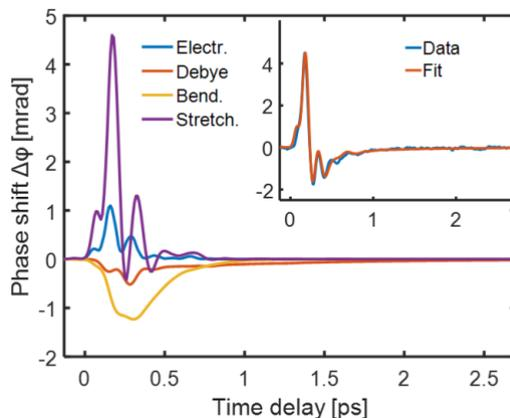
**Figure 15. Simulation of the TKE response.** <sup>[85]</sup> The simulation results of the TKE response in the time domain for the electronic (Electr.), Debye relaxation (Debye), hydrogen bond bending vibration (Bend.) and hydrogen bond stretching vibration (Stretch.) contributions. Inset: a comparison between the sum of all the contributions and the measured data.
