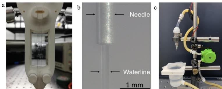
**Figure 2. Liquid targets and the liquid system.** **a** A gravity-driven water film. The thickness is  $210 \mu\text{m}$ . **b** A pump-driven water line with a diameter of  $260 \mu\text{m}$ , which is guided by a syringe needle. **c** A home-built liquid system, which needs only 50 ml water for several hours running. A syringe is used as a jet for producing a liquid line.
