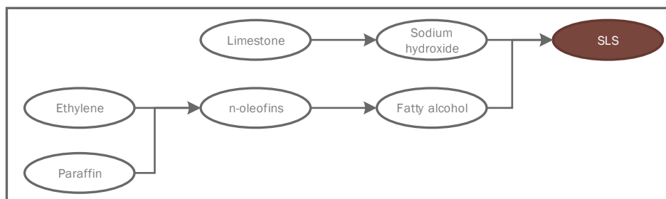
Figure 7.9. Sodium alkyl sulfate production process.
