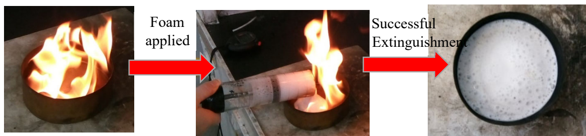
Figure 3. Small scale lab test of extinguishment and foam stability on fire.
