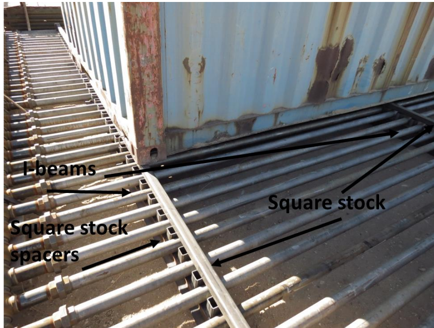
Figure 2-6. The propane burner on an I-beam supporting a large-scale MPPEH surrogate.
