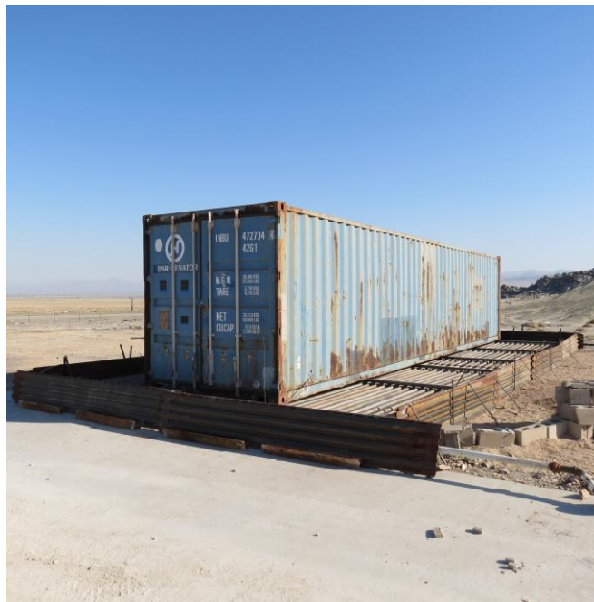
Figure 6-1. Photograph of surrogate for MPPEH on the burner prior to testing at NAWS China Lake.
