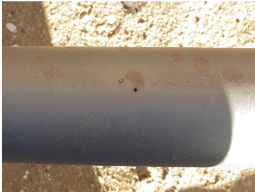
Figure 2-5. Photograph of a single nozzle in a 2 inch burner pipe
