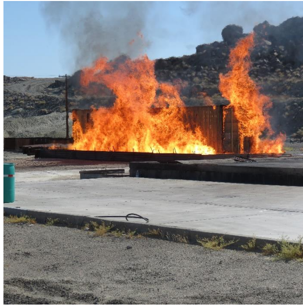
Figure 4. Photograph taken at Naval Air Weapons Station China Lake of large scale flashing of a sea container as a surrogate for MPPEH.
