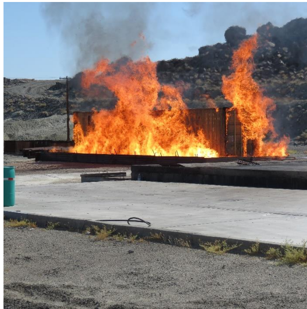
Figure 2-7. Photograph taken at NAWS China Lake of the large-scale flashing of a sea container as a surrogate for MPPEH.
